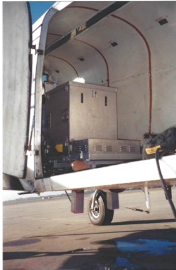
Figure 30: Top: Me sitting in the cockpit of one of the Beech 18s we flew in the Med Fly Project. Officially, these are Hamilton Westwind IIIs, a turbo-prop conversion of the original 1940s-era radial-engine aircraft. Below is a view of the 3-foot-square aluminum box of 6-7 million fruit flies loaded in the back of one of the planes. The machine the box is resting on is both a refrigeration unit to keep the flies lethargic as well as an auger system to push the flies gradually out of the bottom of the plane through the two square chutes visible protruding downward out the bottom of the fuselage.
